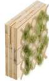
clt shear wall the vertical structure of the residences allows for modular building and layout in addition to vertical growing walls.
